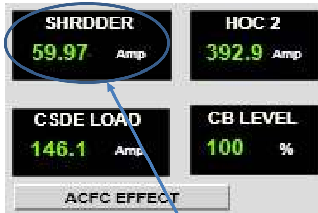
HT MOTOR LOAD 11KV, 100A / 1A HT CT USED FOR CURRENT SENSING
